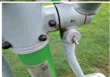
Finding: The buffers are worn or missing, 8 needed
